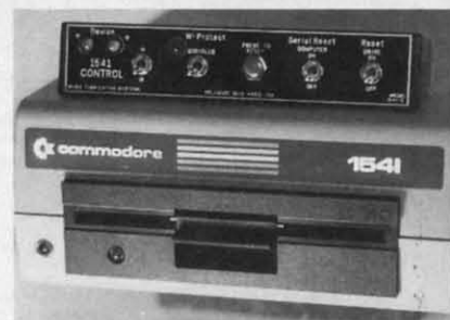
1541 Control: change device #, reset. READER SERVICE NO. 206
